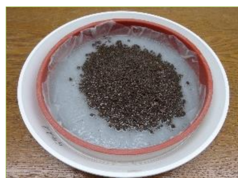
Fig. 4: Water filled sieve tray with 150g of soil
